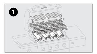
1. Open the top lid. Remove the cooking grates and heat plates to reveal the burners. **Figure 1**
