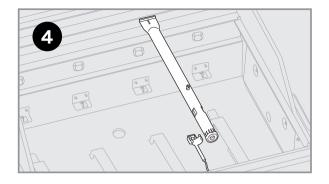
3. When installing your new burners, start with the lighting burner. Attach the electrode clip to the underside of the burner. **Figure 4**
