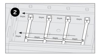
2. Remove the assembly hardware and the carryover assembly for each burner. **Figure 2**
